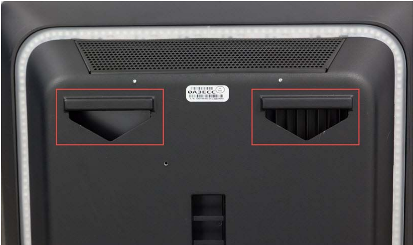
Receptacles on back of jukebox
